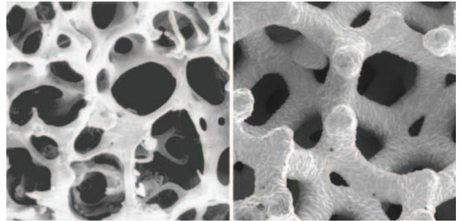
**Figure 1.** SEM view of trabecular bone (left) and Trabecular Metal Material (right).
