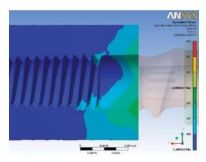
Fig 3. Typical stress distribution in the bone.
