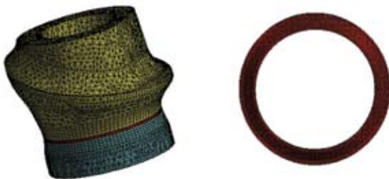
Fig 3. FE mesh for the zirconia abutment and titanium seating ring model.
