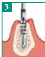
3 FOR SOFT BONE OP3.5D/TLSDS 3.5mmD Drill
